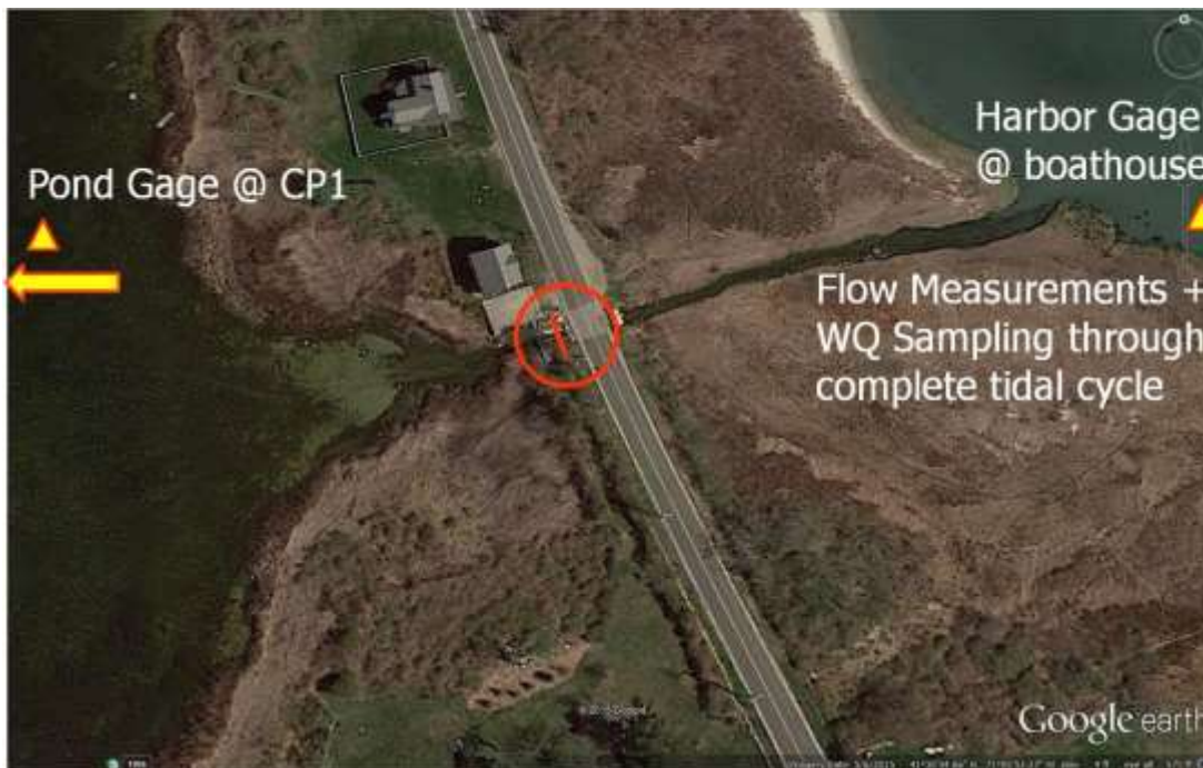
Figure 6. Location of the transect along which velocity measurements and water sampling was conducted for calculation of flow and mass influx/efflux of nutrients in/out of Cockeast Pond.
